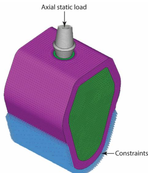
**Figure 3. Representation of the boundary and the loading conditions on the three-dimensional finite element model of the dental implant and the surrounding bones.**
