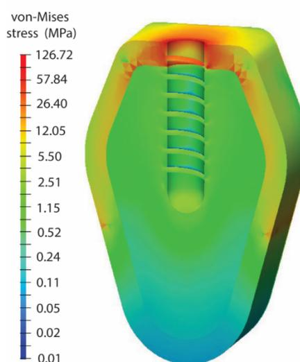
**Figure 4. Distribution of von-Mises stresses within the surrounding bone of the buttress thread implant at 50% osseointegration with the application of axial static occlusal load of 500 N (buccolingual cross sectional view).**
