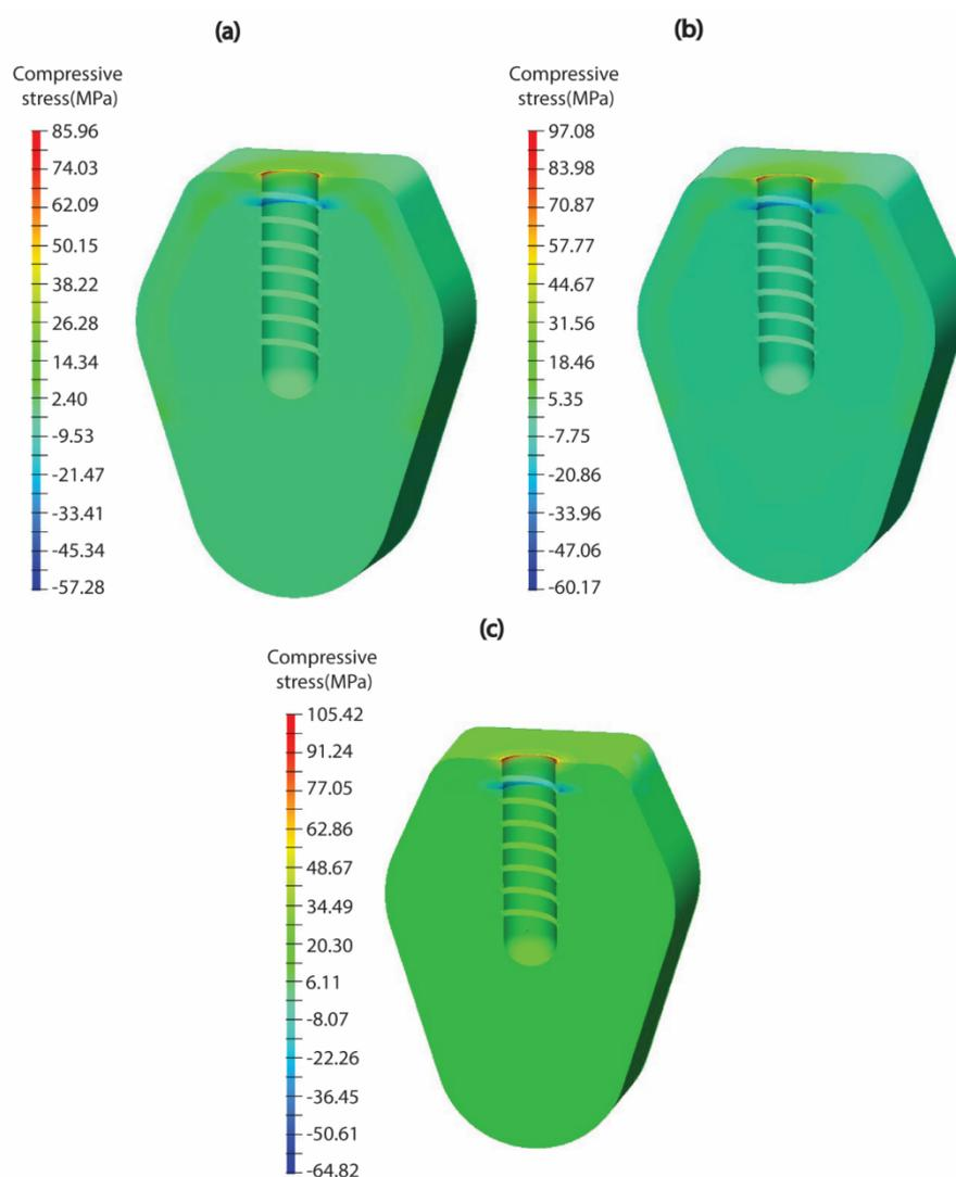
**Figure 6. Distribution of compressive stresses within the surrounding bone of the buttress thread implant with the application of axial static occlusal load of 500 N (buccolingual cross sectional view). (a) 50% osseointegration, (b) 75% osseointegration, and (c) 100% osseointegration.**
