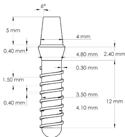
**Figure 1.** Schematic representation of design parameters used for modeling the dental implant and the abutment.
