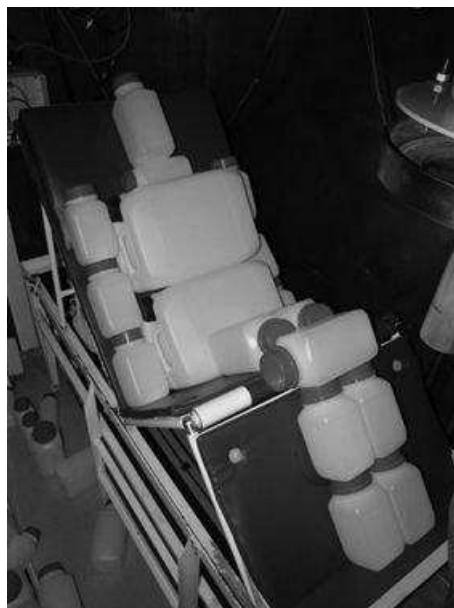
Figure 1. The bottle phantom reproducing the standard human silhouette (70 kg, 170 cm) serving as a calibration phantom at Radiation Protection Measurements Laboratory
