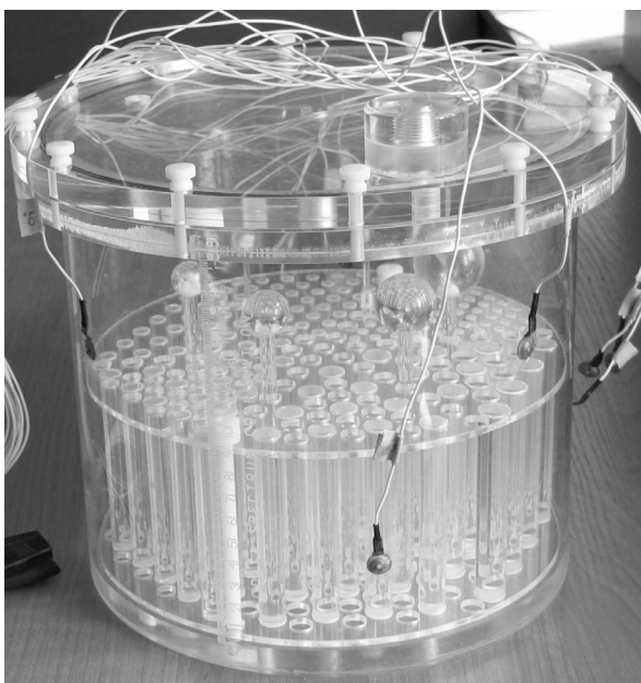
Figure 4. Electrode positions on the Jaszczak phantom: a) eight electrodes marked by Pb spheres, b) three electrodes filled with isotope solution.
