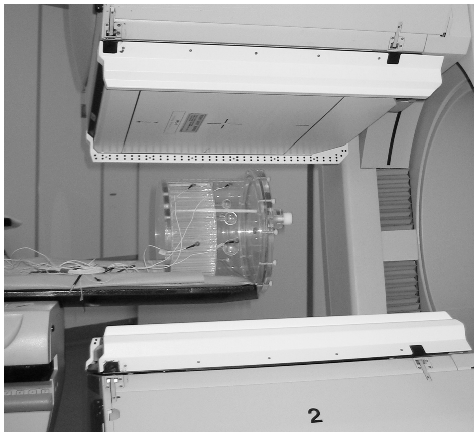
Figure 3. SPECT examination of the Jaszczak phantom with electrodes located on the surface.
