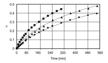
Figure 2. Comparison of computer results (solid lines) with the experimental data (symbols) for the esterification reaction of methacrylic acid with ethanol in the presence of H<sub>3</sub>PMo<sub>12</sub>O<sub>40</sub> (◆ T=348K 1:3 3.12 wt%, ▲ T=348K 1:3 6.24 wt%, ■ T=348K 1:3 12.48 wt%)
