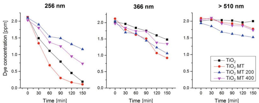
**Figure 7.** Concentration of dye on the exposure time for suspension with photocatalyst by light with different wavelength for raw and modified TiO<sub>2</sub>
