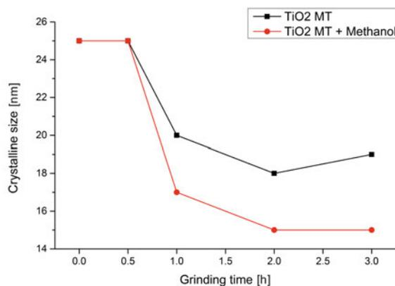
**Figure 3.** Average grain size of  $\text{TiO}_2$  after mechanochemical treatment in air and methanol
