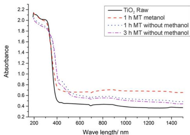
**Figure 5.** UV-Vis diffuse reflectance spectra of pure and subjected to mechanochemical treatment TiO<sub>2</sub>
