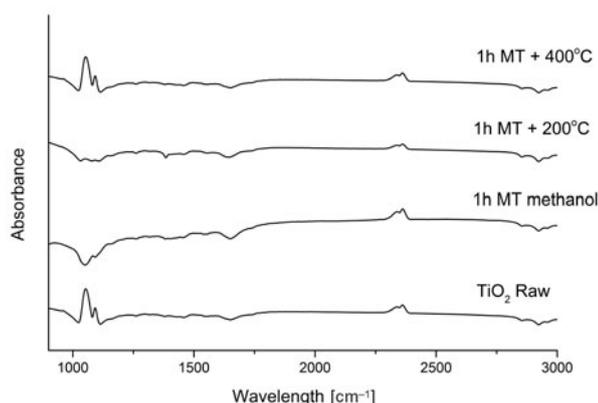
**Figure 4.** IR spectra of raw TiO<sub>2</sub>; powder milling for 1h in methanol and subsequent calcination at 200 and 400°C
