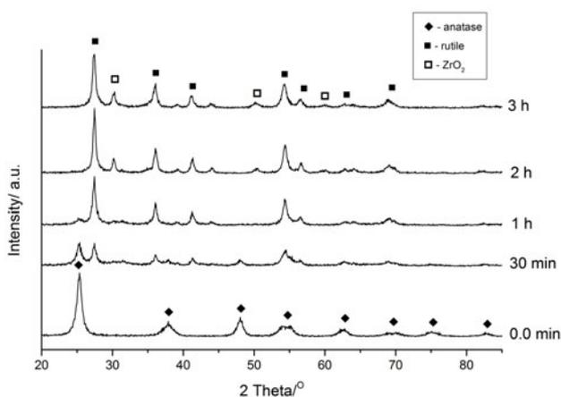
**Figure 1.** X-ray diffraction patterns of  $\text{TiO}_2$  subjected to mechanochemical treatment in air
