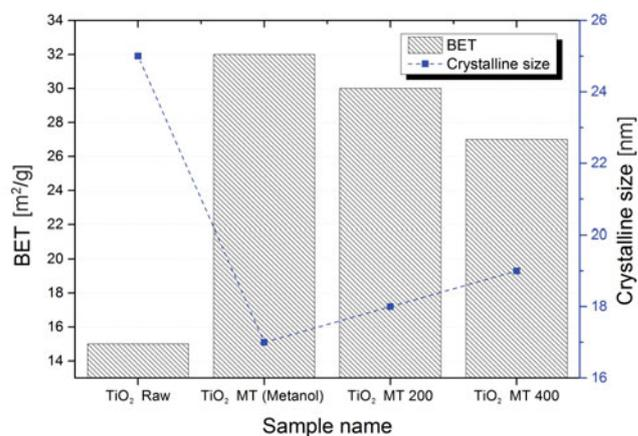
**Figure 6.** BET specific surface area and average crystallite size of the starting and modified TiO<sub>2</sub>
