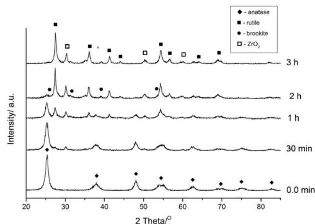
**Figure 2.** X-ray diffraction patterns of  $\text{TiO}_2$  subjected to mechanochemical treatment in the presence of methanol
