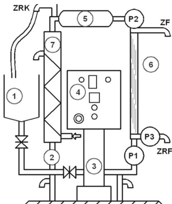
**Figure 1.** Scheme of the UF experimental set-up: 1 – feed tank, 2 – thermometer, 3 – pump, 4 – control panel, 5 – tube furnace, 6 – membrane module, 7 – cooling system, P1, P2, P3 – manometers
