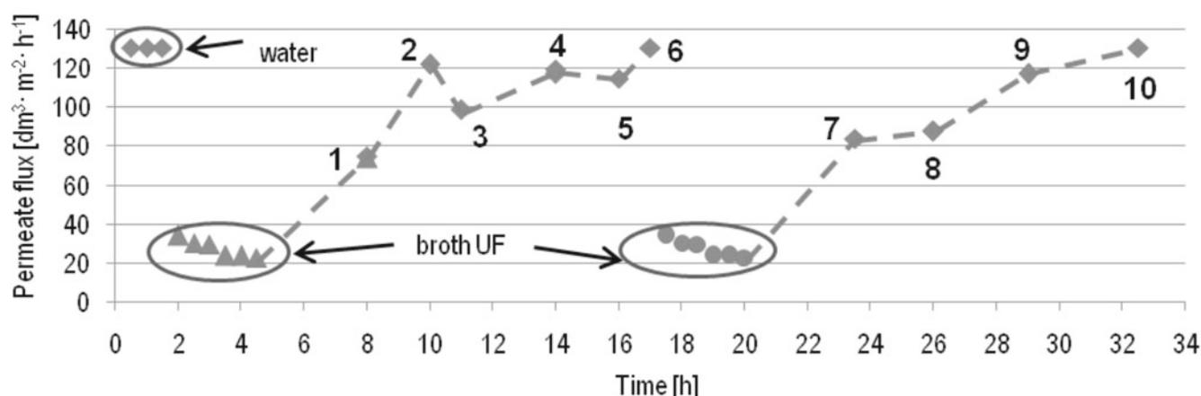
**Figure 2.** Changes of permeate flux versus UF time of the fermentation broth and during the cleaning procedure (membrane cut-off: 15kDa). A dotted line and points 1 to 10- cleaning operation, ▲ – broth I, ● – broth II
