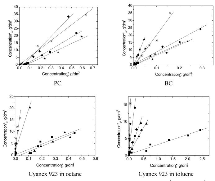
Figure 2. Isotherms of phenol (■), 4-chlorophenol (▲), 2,4-dichlorophenol (▼), 4-fluorophenol (♦), 4-nitrophenol (★), 4-methoxyphenol (●) extraction with various organic phases (Aqueous feed: 0.01 - 22 g/dm<sup>3</sup> of phenols)
