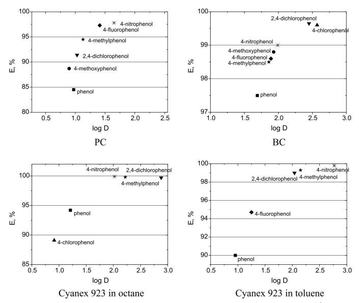
Figure 3. Extraction parameters of selected phenols for Cyanex 923, PC or BC as extractants (Aqueous feed: 1 g/dm<sup>3</sup> of phenol)
