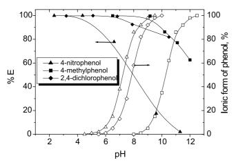
**Figure 4.** Effect of pH change and contribution of ionic form of phenol on extraction efficiency of selected phenols with 0.1 M Cyanex 923
