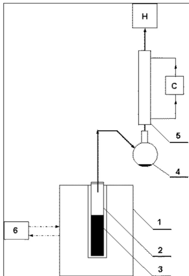
**Figure 4.** Laboratory pyrolytic unit. Notes: 1 – vertical tube oven, 2 – quartz reactor, 3 – pyrolyzed sample, 4 – flask with liquid products, 5 – cooler, 6 – programmable temperature control unit, H – gas holder with gas volume registration, C – cooling unit
