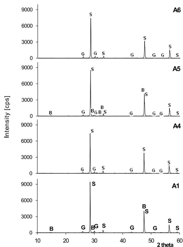
**Figure 2.** X-ray powder diffraction patterns of some leached Zn-concentrate samples (B – bassanite (CaSO<sub>4</sub>·0.5H<sub>2</sub>O), G – galena (PbS), S – sphalerite (ZnS))
