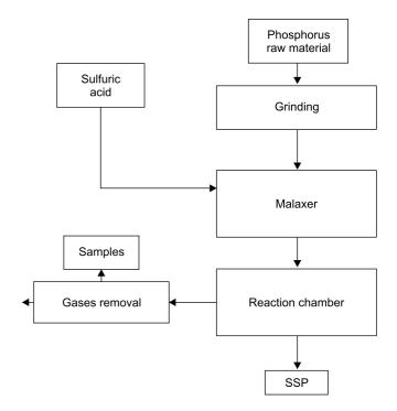
Figure 2. Collecting samples of gases emitted in a single superphosphate production process
