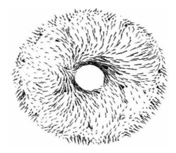
Figure 7. Radial speed in the annular section of the apparatus for  $\phi = 10\%$ ; l = 2mm
