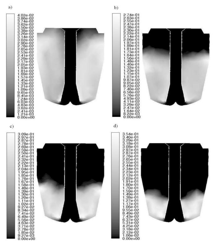
Figure 5. The influence of size of crystallites on the deposit of the fluidal-bed crystallizer for  $\varphi = 10$ ; a) l = 1mm; b) l = 2mm; c) l = 3mm; d) l = 4mm
