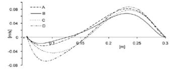
Figure 3. Comparison of solution velocity profiles in the A-A cross-section for different internal crystallizer configurations (the second position of the central tube, the inlet solution velocity 0.61 m/s; the outer wall of the central tube corresponds to x = 0.06 m)
