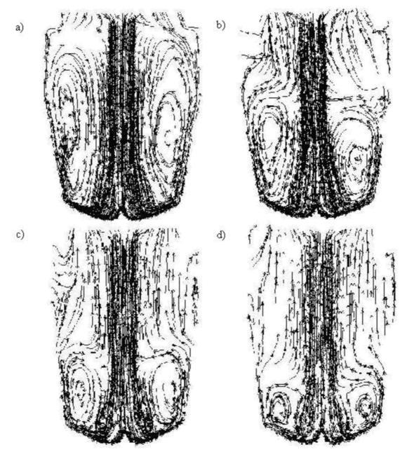
Figure 8. The schedule of the internal circulations of suspension for  $\varphi = 10$ ; a) l = 1mm; b) l = 2mm; c) l = 3mm; d) l = 4mm
