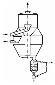
Figure 1. A scheme of the Oslo fluidized-bed crystallizer with the classification leg<sup>16</sup>
