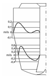
Figure 6. Profiles of axial speeds in the transverse section of the apparatus for  $\phi = 10\%$ ; l = 2mm
