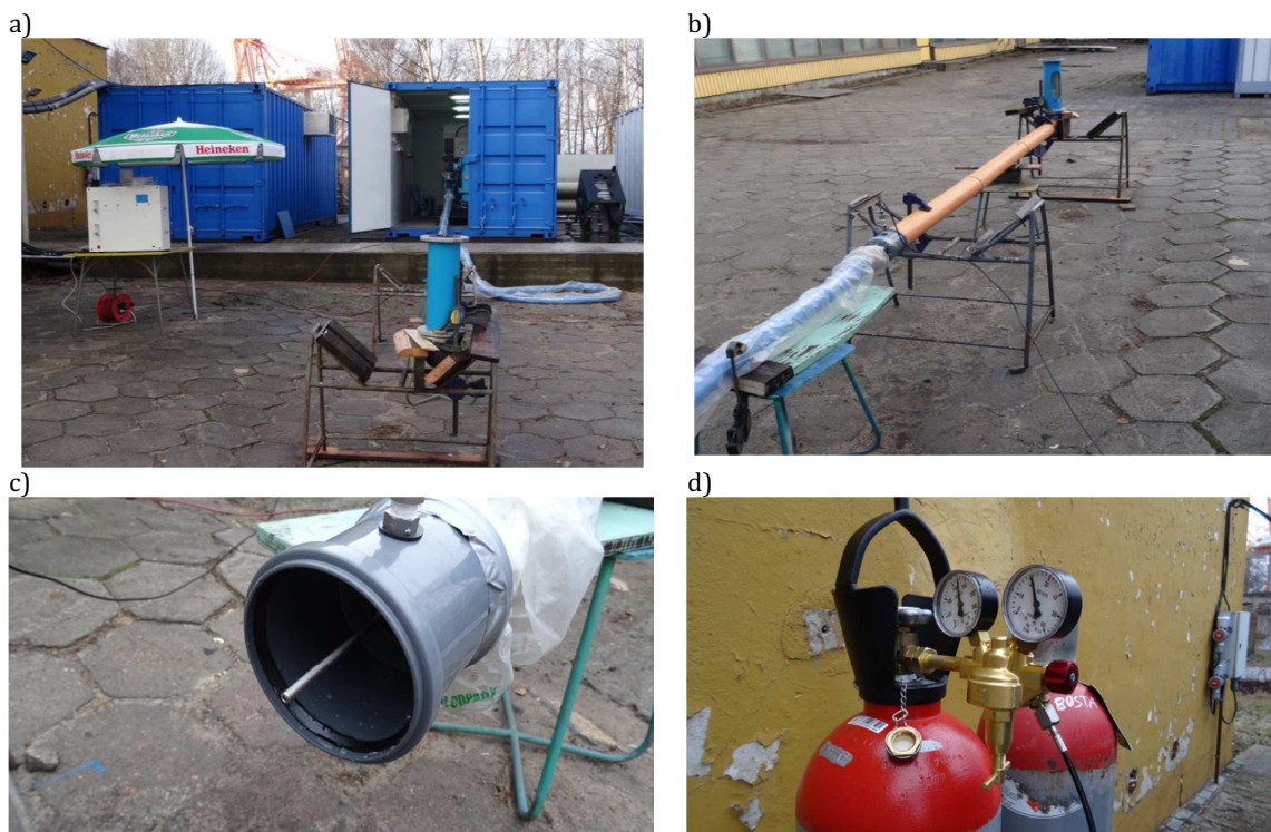
Fig. 9. A Tubular reactor for the production of a hydrogen-air mix: a) view of the air pump station located in the container, the rotametric measurement station is visible from the front; the station of hydrogen content measurement in the air is on the left; b) view of the pipe mixer; the connection of the pumping hose to the dosing head of the tubular reactor is visible closer to the reactor's inlet; c) view of the hydrogen line connection and hydrogen dosing tube to the tubular reactor; inside the hidden casing of the dosing nozzle; d) pressure regulator on the hydrogen supply .
