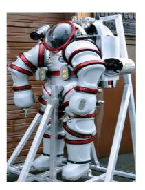
Fig. 1.11. Exsosuit – one-atmosphere diving suite (armoured suite) manufactured by a Canadian company – Nuytico Research Ltd. from North Vancouver [22b].
