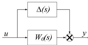
Fig. 2. Decomposed diagram of the control object
