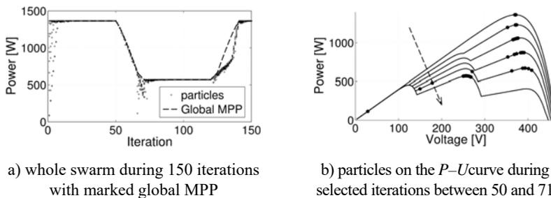
Fig. 9. Numerical results in the fourth test scenario (faster change in irradiance than in the third scenario)
