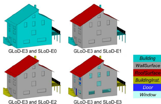
Fig. 5: Combining geometric LoD and semantic LoD in CityGML (Benner et al. 2013).
