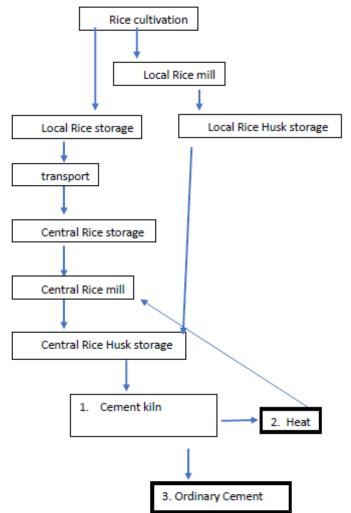
*Figure 3 – Scenario 3, Rice husk as fuel in a rotary kiln for cement production.*
