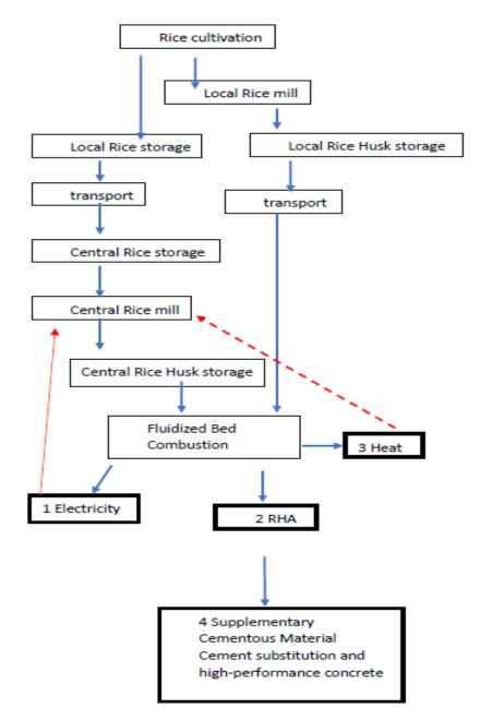
Figure 2 – Scenario 2 Product system for production of Energy and RHA and as a SCM.
