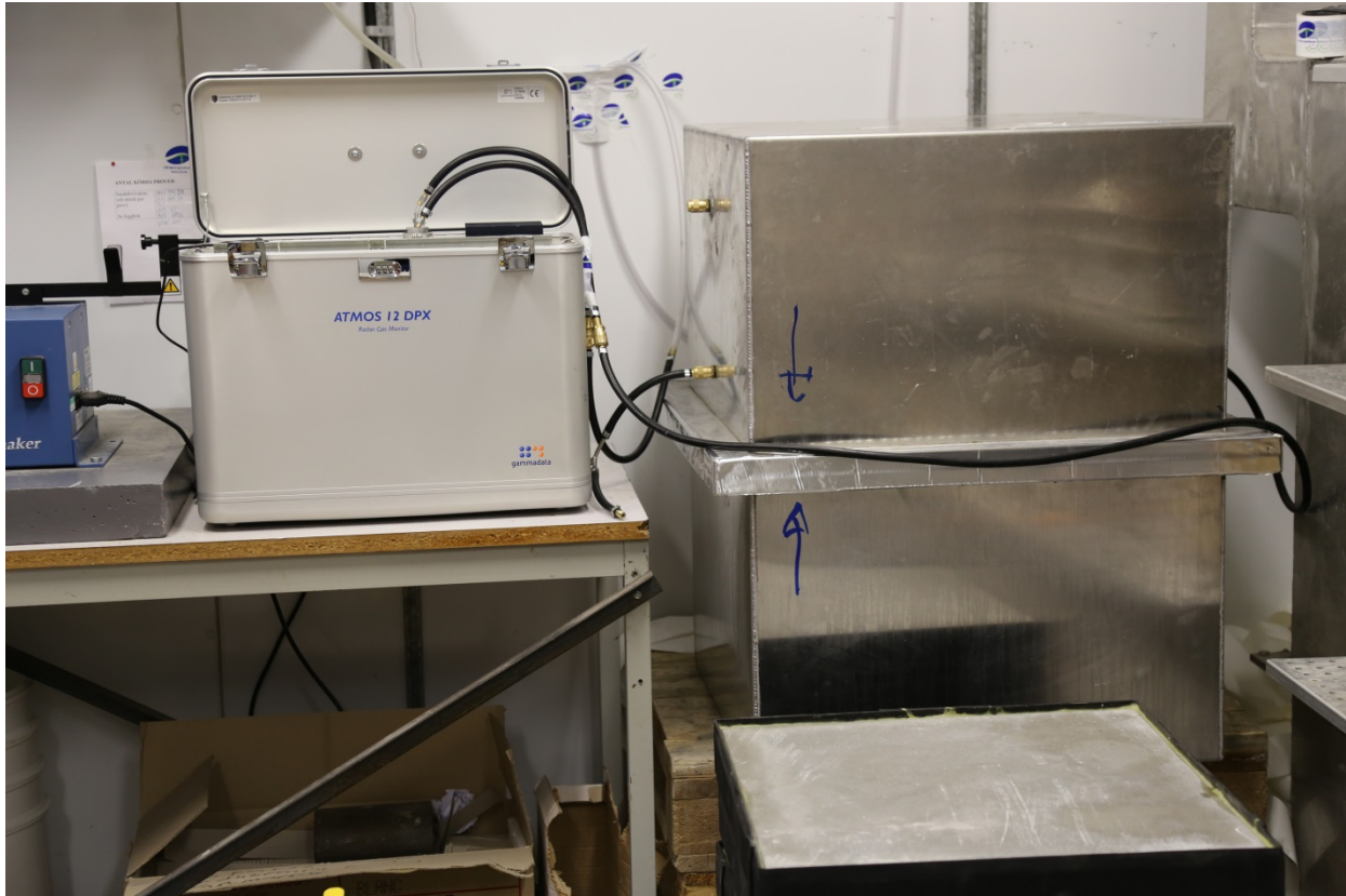
Figure 2 – The Atmos 33 (Atmos 12DPX) connected to the aluminum container. The hoses and connectors used are intended for high pressure gas flow (welding equipment). They are used as to ensure no leakage. The sealing of the containers is made with a butyl-aluminum tape that has been tested to ensure no leakage of radon.
