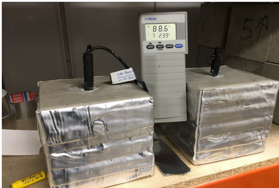
Figure 3 – Two of the three investigated concrete cubes (150 X 150 X 150 mm) sealed with aluminum tape on each side except the top. The figure also shows the plastic tubes on top as to measure the relative humidity. The current reading is 88.6 % in relative humidity using probe 7 at 23.9°C for the recipe containing an additive.
