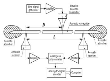
Fig.1 Ultrasonic interferometric encoder of distance.
