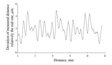
Fig.2 A typical deviation chart of measured distance in relation to the real one.
