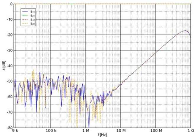
Fig.2 Measured scattering parameters of realised coaxial flange
