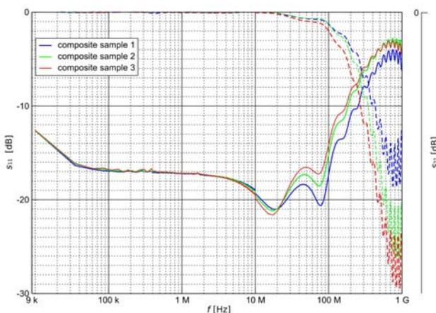
Fig.6 Scattering parameters of tested composite materials (s<sub>11</sub> - full lines, s<sub>21</sub> - dashed lines)
