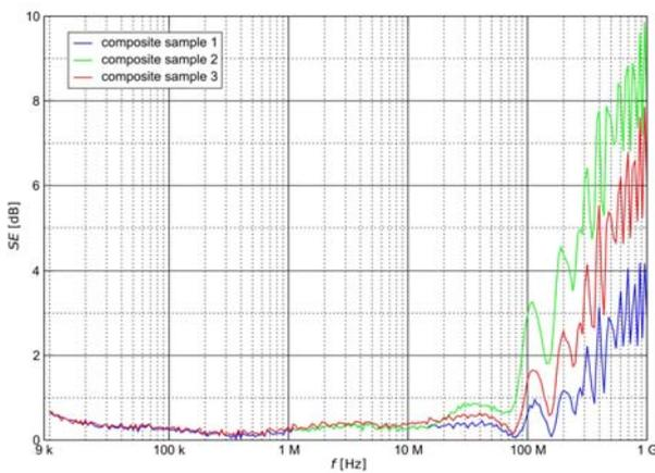
Fig.5 Shielding efficiency of the composite materials
