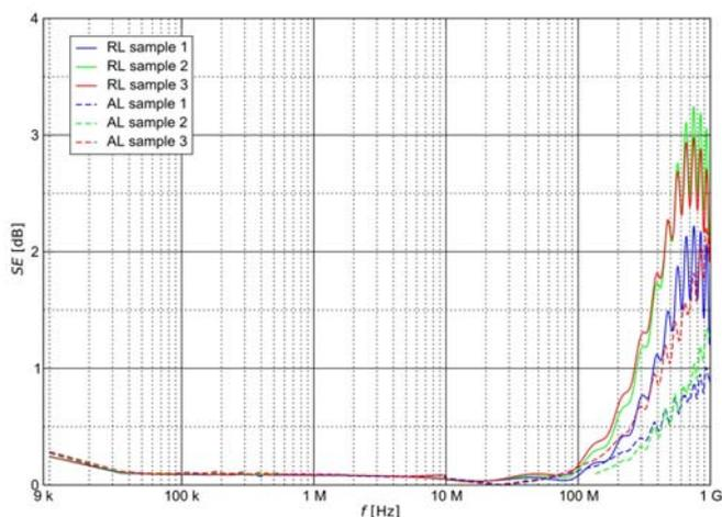
Fig.7 Calculated shielding efficiency components (reflection and absorption losses )
