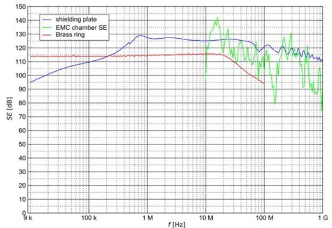
Fig.3 Performance comparison of the shielding measurement methods
