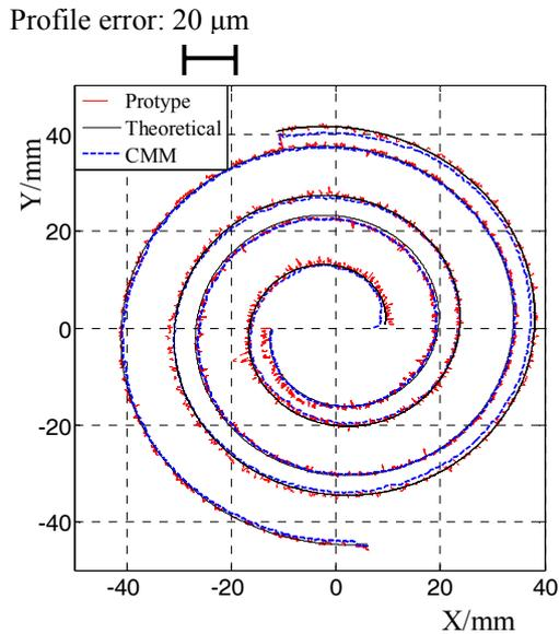
Fig.6 Measurement results for involutes profile of scroll
