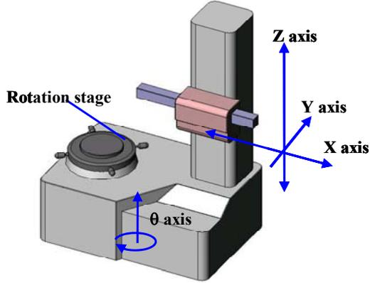
Fig.2 Measurement system of scroll profile
