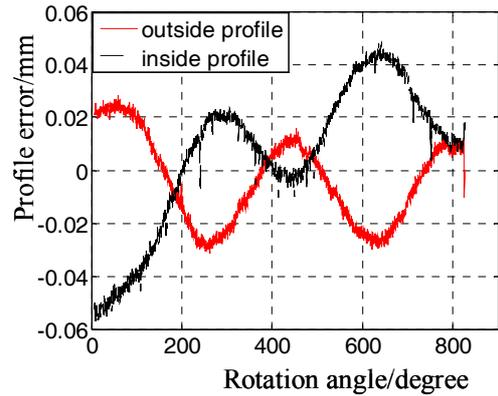
Fig.3 Measurement result without error separation
