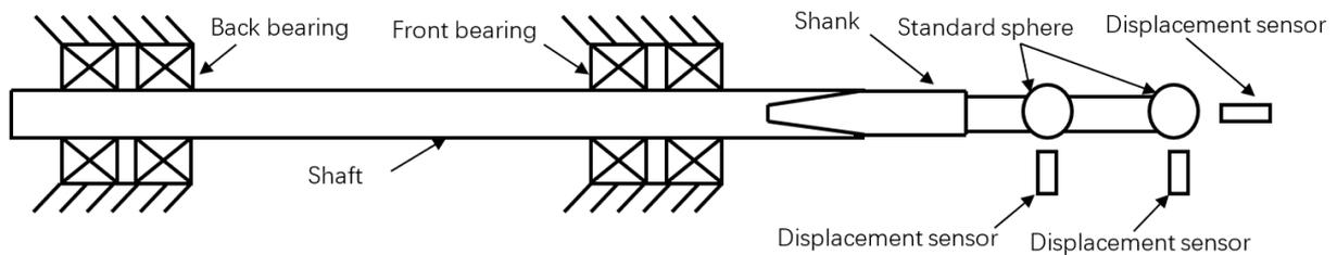
Fig. 15. Principle of the spindle vibrations detection.
