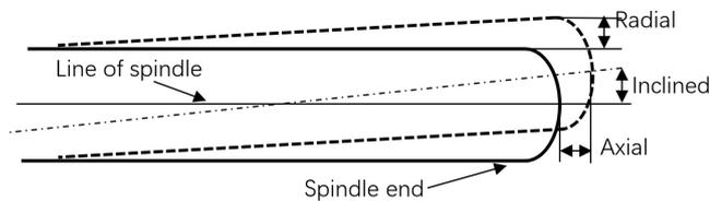
Fig.1. Schematic diagram of spindle vibrations.
