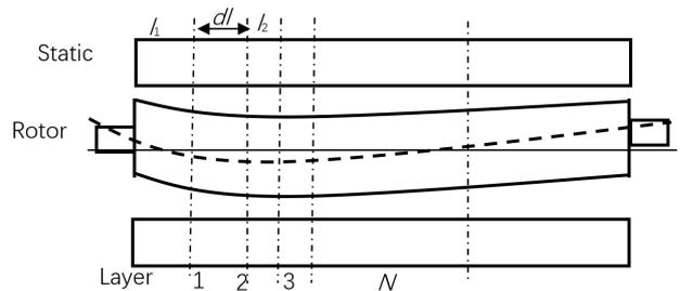
Fig.7. Schematic diagram of the curved eccentricity.
