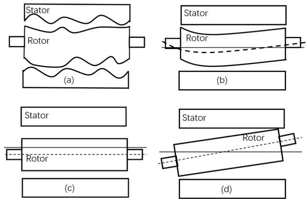
Fig.2. The main mechanical sources of air-gap eccentricity: a) shape deviation, b) parallel eccentricity, c) inclined eccentricity, and d) curved eccentricity.
