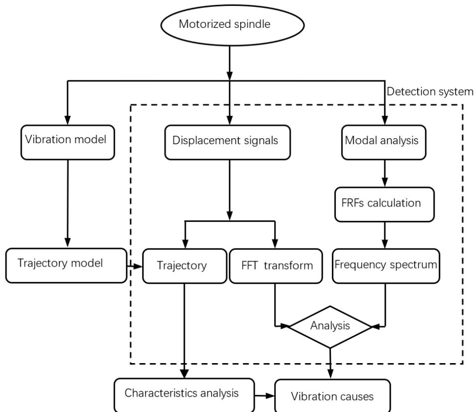
Fig. 16. Flow chart of the spindle vibrations detection.
