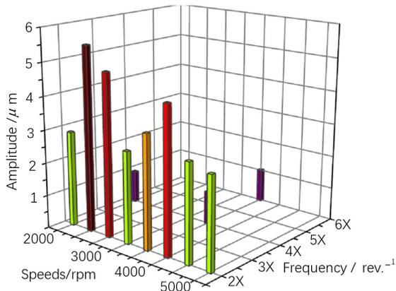
Fig.21. Measured vibration signals spectrum.
