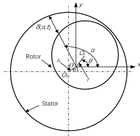
Fig.4. Schematic diagram of static and dynamic mixed eccentricity.
