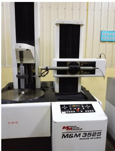
Fig.11. Gear measurement center.
