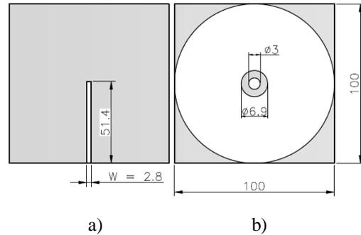
Fig.3. a) Strip side and b) ground plane side of proposed planar coaxial probe (unit: mm).
