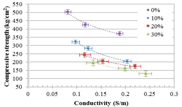
Fig.12. Relationship between compressive strengths and conductivities of concrete with different percentages of RHA at frequency of 3.2 GHz.
