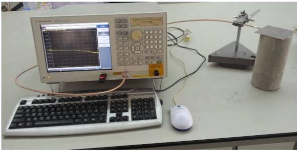
Fig.4. Measurement setup for investigating dielectric properties of concrete specimens.
