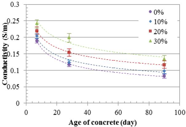
Fig.10. Conductivities of concrete with different percentages of RHA at frequency of 3.2 GHz versus concrete age.
