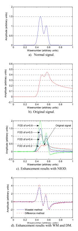
Fig.8. NIOD for signal enhancement and its comparison with WM and DM
