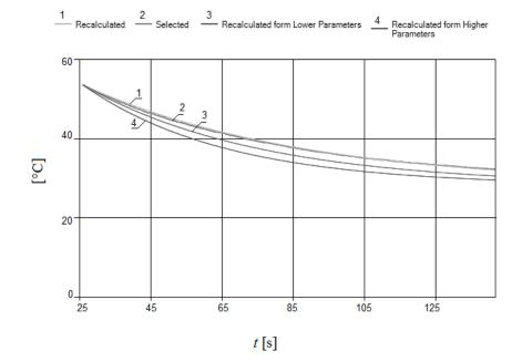
Fig.3. Print screen of a relatively good estimate shows a window enabling to track the difference between the experimental curve and the curves calculated from the top and bottom estimates of  $h_t$ , k,  $c_p$ , and  $\alpha$  (colors of curves are not distinguished in the picture).
