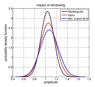
Fig.3. PDF of the field amplitude M at 24.41 MHz for different time windows. The spread and the bias increase with the *ENBW* of the selected window.
