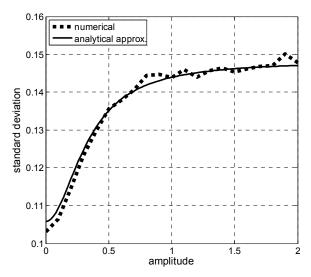
Fig.5. Analytical vs numerical behavior of the standard deviation of the simulated noisy field at 24.41 MHz. Noise levels and sampling conditions are the same as in Fig.2.
