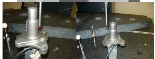
Fig.7. Measurements performed on: simulator and Leitz PMM 12106 machine.
