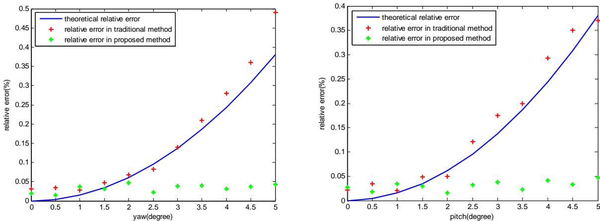
Fig.8. Relative errors of the speed estimation with yaw and pitch changing.
