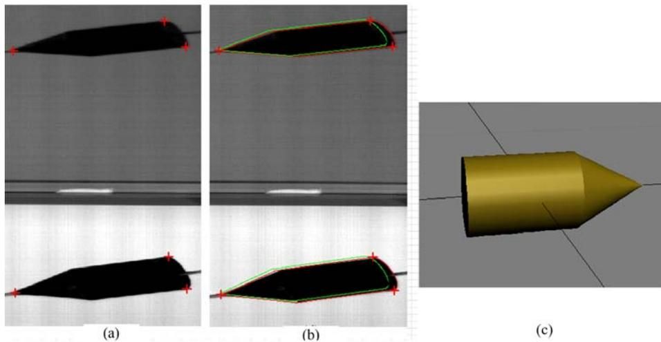
Fig.6. (a) stereo image and special points; (b) the stereo projections related to the initial and the optimal estimation results; (c) 3D model of reduced scale model.
