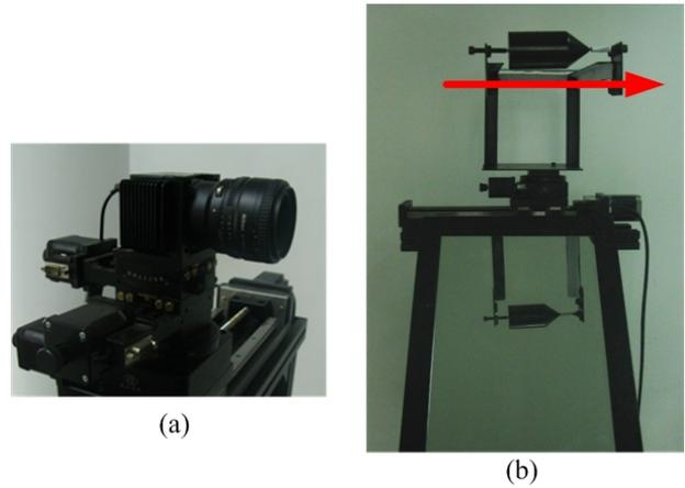
Fig.5. (a) digital line-scan camera(BASLER spL2048-140km); (b) moving reduced scale model target and its reflection in the mirror.
