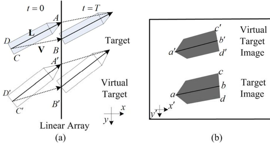
Fig.2. (a) The displacement of the target and its virtual counterpart in space (seen in the direction of the axis  $z$ ); (b) stereo images of the target.
