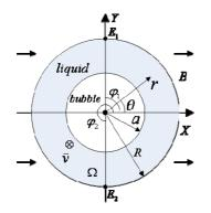
Fig.3. The electrodes section diagram of EM flow-meter
