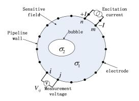
Fig.1. Schematic diagram of ERT sensor
