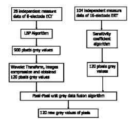
Fig.7. The diagram of data fusion process
