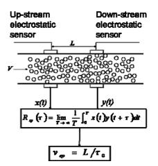
Fig.13. The diagram of correlation operation
