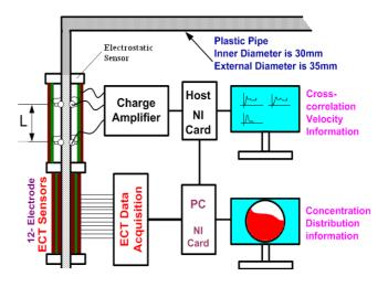
Fig.8. The fusion system of ECT with Electrostatic sensors
