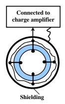
Fig.10. The section diagram of electrostatic sensor
