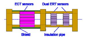
Fig.4. Fusion sensor of ECT sensors with dual ERT sensors
