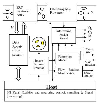
Fig.2. The diagram of the whole measuring system
