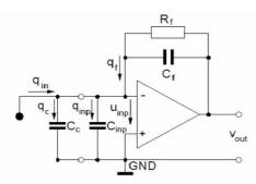
Fig.11. The diagram of charge amplifier
