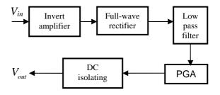
Fig.12. The diagram of further signal processing
