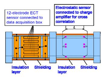
Fig.9. The diagram of ECT and electrostatic sensors
