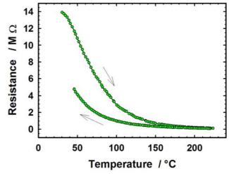
Fig.2. R vs. T dependence of the 100 min milled and by 200 MPa pressed sample. (The arrows show the increase and following decrease of temperature).
