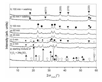
Fig.1. XRD patterns of the starting  $V_2O_5 + 2Na_2SO_3$  mixture (a), and powders milled between 2 and 100 min (b-h). ( $\blacktriangle$ ):  $V_2O_5$ , ( $\blacktriangledown$ ):  $VO_2$ , ( $\circ$ ):  $Na_2SO_3$ , ( $\bullet$ ):  $Na_2SO_4$ , ( $\blacksquare$ ):  $VO_2$ :  $xH_2O$ .
