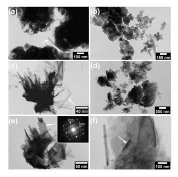
Fig.4. TEM images of VO<sub>2</sub> obtained by milling of the  $V_2O_5 + 2$  Na<sub>2</sub>SO<sub>3</sub> mixture for 5 min (a), 20 min (b), 60 min (c) and 100 min (d-f) after the subsequent washing procedure.
