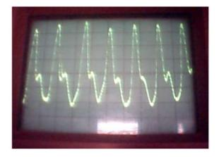
Fig.4. Oscilloscope view of optical sensor measurements after conditioning circuit
