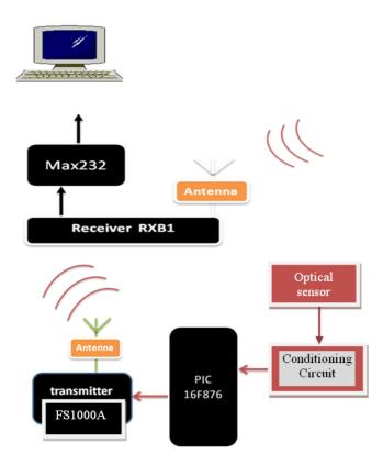
Fig.2. Block diagram of the data-acquisition system.
