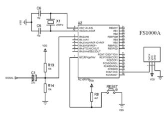
Fig.5. The processing card with high frequency transmission
