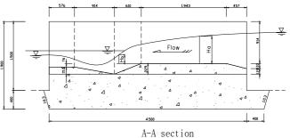
Fig.1. The designed Parshall flume
