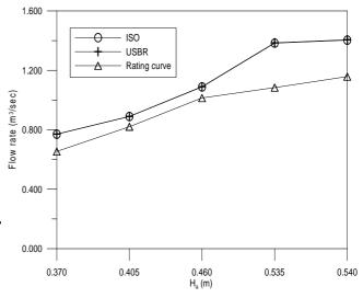
Fig.4. The comparison of flow rates computed by Parshall flume equation and rating curve.
