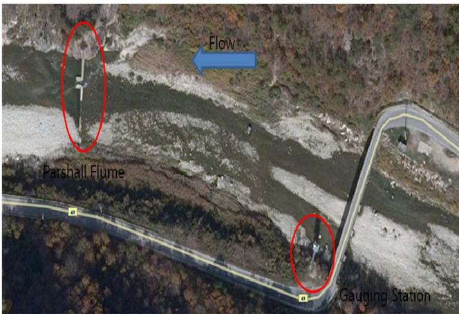
Photo 1. Parshall flume, gauging station and catchment
