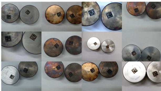
**Fig. 2 Data Matrix code samples laser-marked in metal**
