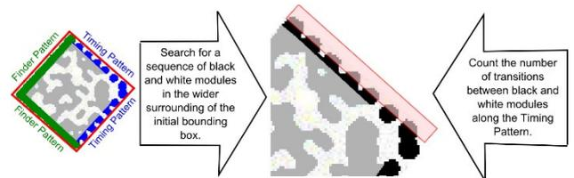
**Fig. 3c Flowchart for the third phase: verification of Timing Patterns of Data Matrix code**
