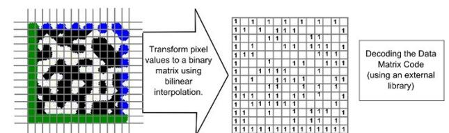
**Fig. 3d Flowchart for the last phase: decoding of Data Matrix code**
