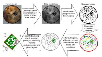
Fig. 3a Flowchart for the first phase: raw location of Data Matrix codes in images
