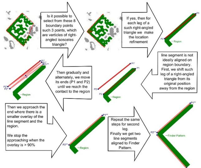
**Fig. 3b Flowchart for the second phase: location of Finder Patterns of Data Matrix code**
