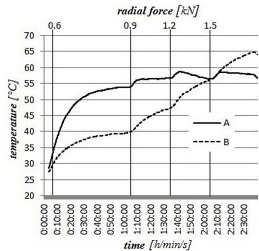
**Fig. 3** The course of average temperature in the particular bearing A and B
