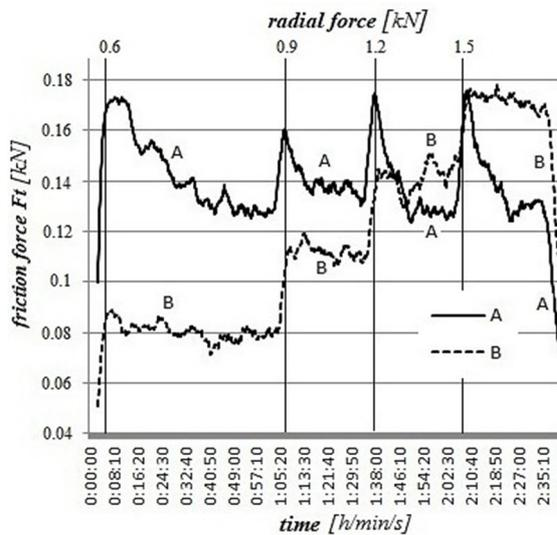
**Fig. 2** The course of average frictional forces in the bearing A and B
