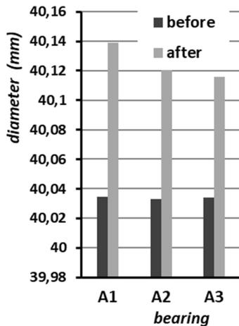
**Fig. 5** The average values of the diameter of the bearings A before and after the experiment
