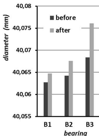
**Fig. 6** The average values of the diameter of the bearings B before and after the experiment
