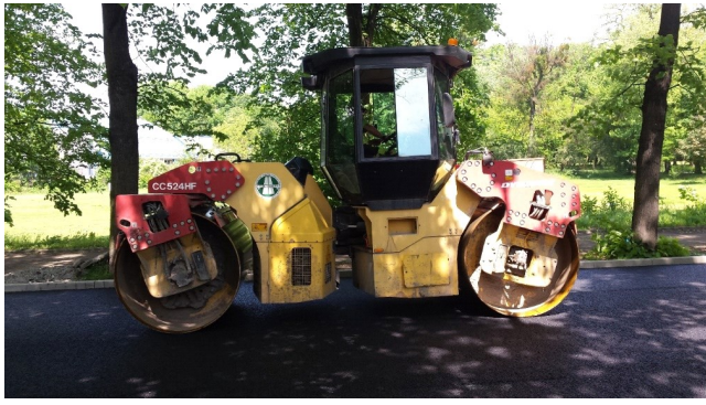
Fig. 1 Two-shaft road roller type Dynapac CC524HF Source: Own photo.
