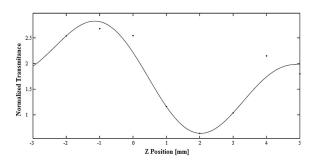
Fig. 4. Closed aperture Z-Scan data for Para Red solution.
