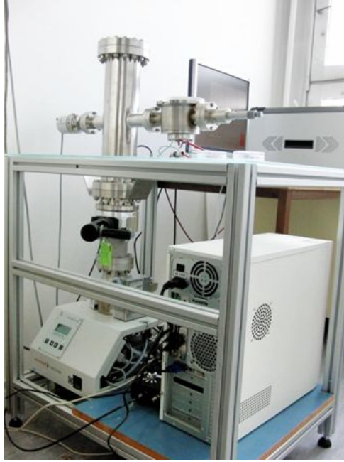
Fig. 1. The experimental chamber setup for FE measurements. This experimental setup is equipped with vacuum pump; vacuum vessel; experimental vacuum chamber; vacuum measuring head; high voltage supply; computer for data acquisition and analysis.
