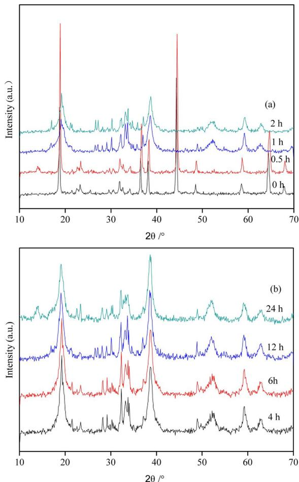
Fig. 4. XRD patterns of samples prepared at different grinding times (a) 0 h to 2 h samples and (b) 4 h to 24 h samples.
