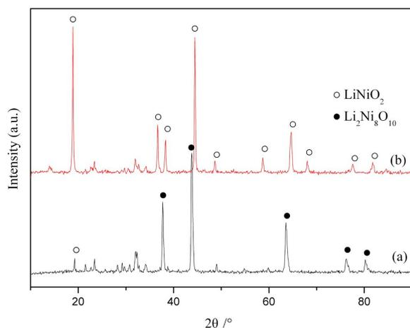
Fig. 2. XRD patterns of the products originating from (a)  $\text{Li}_2\text{CO}_3 + \text{Ni}(\text{OH})_2 \cdot \text{H}_2\text{O}$  and (b)  $\text{LiOH} \cdot \text{H}_2\text{O} + \text{Ni}(\text{OH})_2 \cdot \text{H}_2\text{O}$ .
