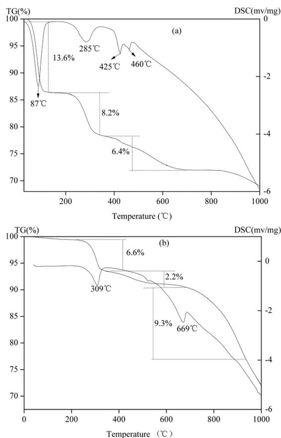
Fig. 1. TG-DTA curves of starting materials (a)  $\text{LiOH}\cdot\text{H}_2\text{O} + \text{Ni}(\text{OH})_2\cdot\text{H}_2\text{O}$ , (b)  $\text{Li}_2\text{CO}_3 + \text{Ni}(\text{OH})_2\cdot\text{H}_2\text{O}$ .
