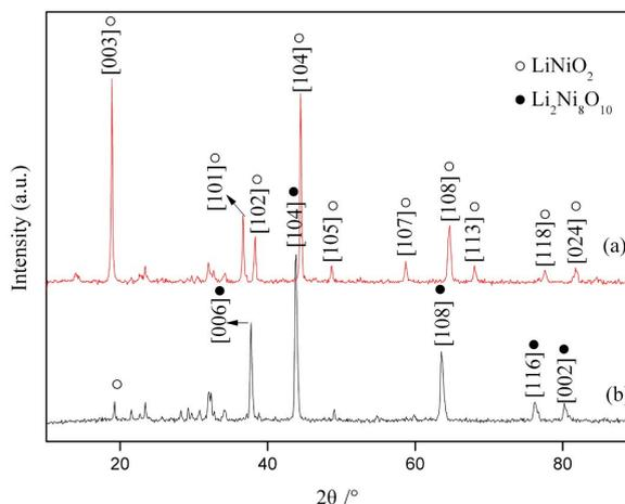
Fig. 3. XRD patterns of samples obtained at different grinding speeds (a) 580 rpm and (b) 400 rpm.
