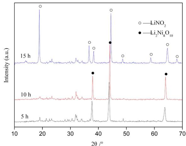
Fig. 5. XRD patterns of samples prepared by heat treatment for different time periods.
