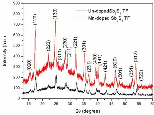
Fig. 1. The XRD patterns for undoped and Mn-doped Sb<sub>2</sub>S<sub>3</sub> TFs.
