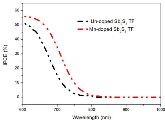
Fig. 7. The IPCE spectra of undoped and Mn-doped  $\text{Sb}_2\text{S}_3$  TFs attached to  $\text{TiO}_2$  NWs.
