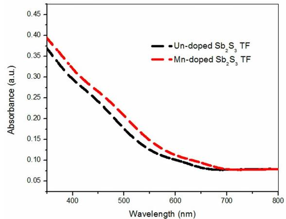
Fig. 2. The optical absorbance spectra of undoped and Mn-doped Sb<sub>2</sub>S<sub>3</sub> TFs.
