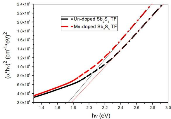
Fig. 3. Determination of the optical band gap for the undoped and Mn-doped  $\text{Sb}_2\text{S}_3$  TFs using  $(\alpha h\nu)^2$  vs.  $h\nu$  plot.
