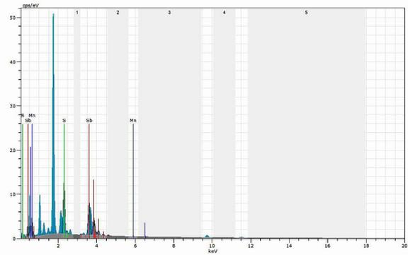
Fig. 5. EDX spectrum of the Mn-doped  $Sb_2S_3$  TF synthesized at room temperature.
