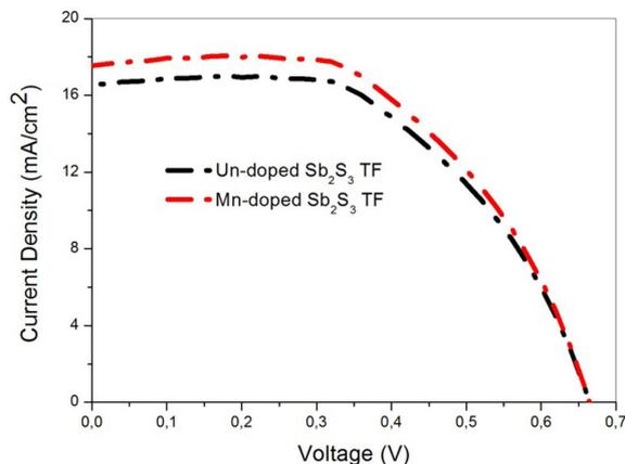
Fig. 8. J-V plots of undoped and Mn-doped  $\text{Sb}_2\text{S}_3$  TFs attached to  $\text{TiO}_2$  NWs.
