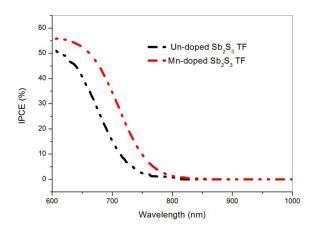
Fig. 7. The IPCE spectra of undoped and Mn-doped  $Sb_2S_3$  TFs attached to TiO<sub>2</sub> NWs.
