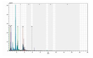
Fig. 5. EDX spectrum of the Mn-doped Sb<sub>2</sub>S<sub>3</sub> TF synthesized at room temperature.
