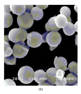
Fig. 4. SEM images of (a) undoped  $Sb_2S_3$  TF, (b) Mn-doped  $Sb_2S_3$  TF.
