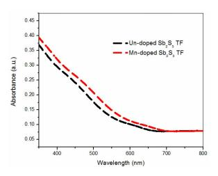
Fig. 2. The optical absorbance spectra of undoped and Mn-doped  $Sb_2S_3$  TFs.
