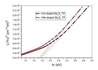
Fig. 3. Determination of the optical band gap for the undoped and Mn-doped  $Sb_2S_3$  TFs using  $(\alpha h \upsilon)^2$  vs. h $\upsilon$  plot.
