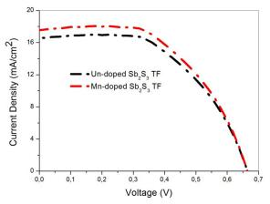
Fig. 8. J-V plots of undoped and Mn-doped  $Sb_2S_3$  TFs attached to TiO<sub>2</sub> NWs.
