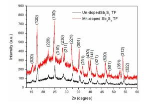
Fig. 1. The XRD patterns for undoped and Mn-doped  $Sb_2S_3$  TFs.
