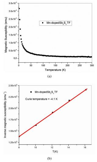
Fig. 6. (a) Magnetic susceptibility versus temperature, (b) inverse magnetic susceptibility vs. temperature for the Mn-doped  $Sb_2S_3$  TF prepared by the CBD method at room temperature.
