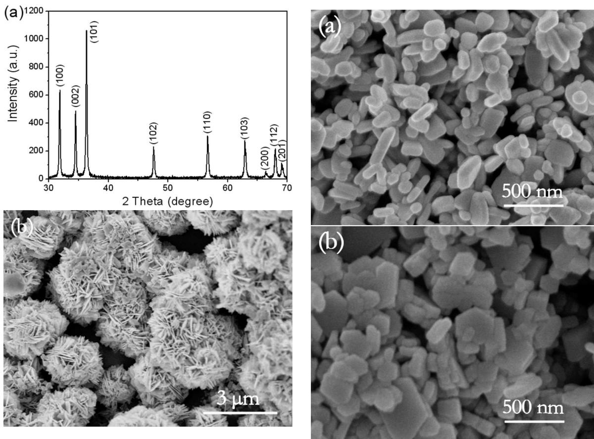
Fig. 1. Characterization of the ZnO samples obtained at pH of the reaction solution of 13.8: (a) XRD pattern and (b) SEM image.
