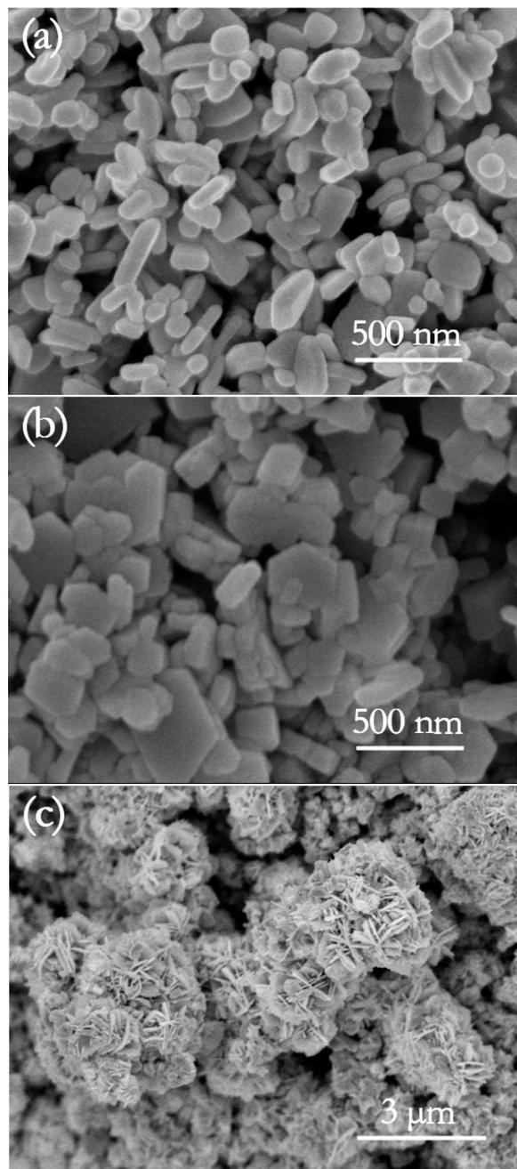
Fig. 2. SEM images of ZnO samples obtained at different pH values of the reaction solutions: (a) 13.1, (b) 13.6, (c) 13.7.
