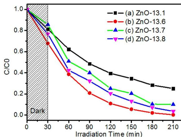
Fig. 4. Photocatalytic performance of ZnO based photocatalysts for degrading MB; the ZnO nanocrystals were obtained at different pH values of the reaction solutions: (a) 13.1, (b) 13.6, (c) 13.7, (d) 13.8.
