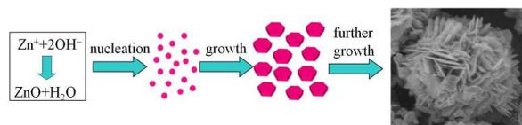
Fig. 3. Illustration of a possible growth mechanism of the ZnO microflowers.
