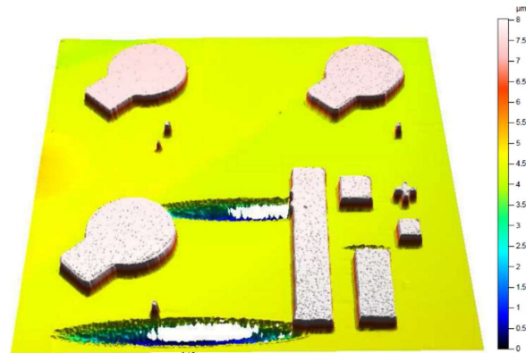
Fig. 8. WLI measurement result after 5 minute etching in 1HCl:1CH 3 COOH:1H 2 O 2 solution.
