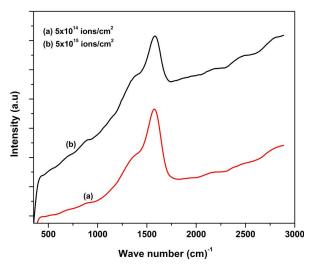
Fig. 3. Raman spectra of 400 keV Au<sup>+</sup> ion implanted CR-39 at (a)  $5 \times 10^{14}$  ions/cm<sup>2</sup> and (b)  $5 \times 10^{15}$  ions/cm<sup>2</sup>.
