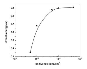
Fig. 10. Urbach energy vs. ion fluence for 400 keV Au<sup>+</sup> ion implanted CR-39.
