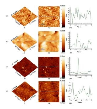
Fig. 5. Surface topography AFM images  $(2 \ \mu m \times 2 \ \mu m)$ of (a) pristine CR-39 and implanted by 400 keV Au<sup>+</sup> ions at (b)  $5 \times 10^{13} \ ions/cm^2$  (c)  $5 \times 10^{14} \ ions/cm^2$  (d)  $5 \times 10^{15} \ ions/cm^2$ . The images on the left hand side of the figure are three-dimentional AFM micrographs, twodimentional topographic scans are in the middle, while line profiles of surface, highlighted in the 2D images, are shown on the right hand side of the figure.
