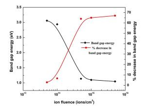
Fig. 8. Plot of optical band gap energy  $(E_g)$  and % decrease in band gap energy vs. ion fluence.
