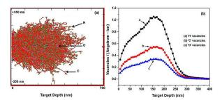
Fig. 1. SRIM/TRIM simulation for 400 keV Au<sup>+</sup> ion implantation in CR-39 (a) estimated ion trajectories (b) vacancies-depth distribution.
