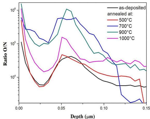
Fig. 4. SIMS depth distributions of O/N ratio for as deposited and annealed films at temperatures 500 °C, 700 °C, 900 °C and 1000 °C.
