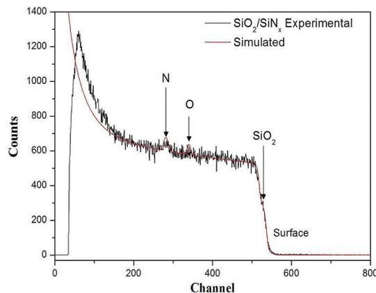
Fig. 5. Typical RBS spectrum of ON structure recorded with  $\text{He}^{+2}$  ions at 2 MeV. Simulation by SIMNRA is given for comparison. Chemical symbol arrows are given to show the signal of each element located at the film surface.
