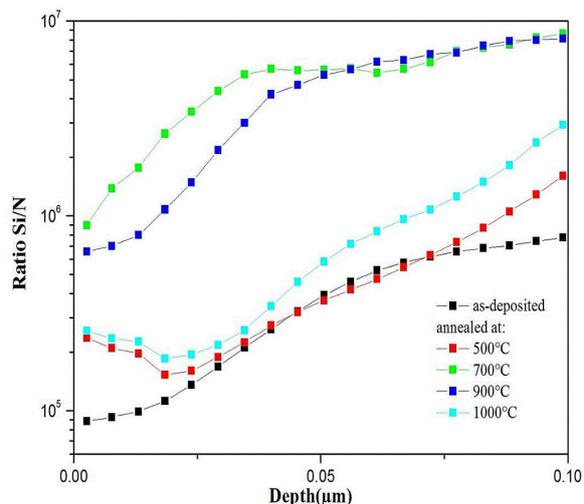
Fig. 3. SIMS depth distributions of Si/N ratio on ON structure for as-deposited and annealed at: 500 °C, 700 °C, 900 °C and 1000 °C.
