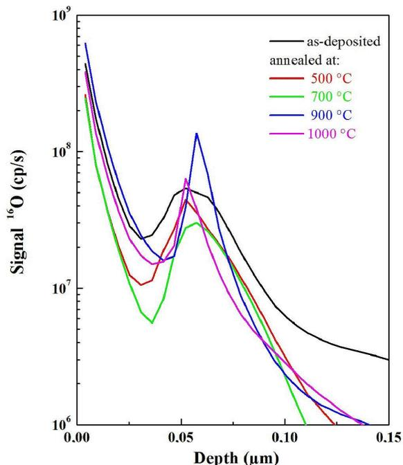
Fig. 2. SIMS depth distribution of oxygen concentration for samples annealed at different temperatures.
