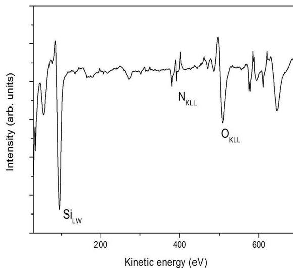
Fig. 6. First derivative AES survey spectrum of oxide/nitride film obtained after dry oxidation of  $\text{SiN}_x$  and annealed at 700 °C during 30 min.
