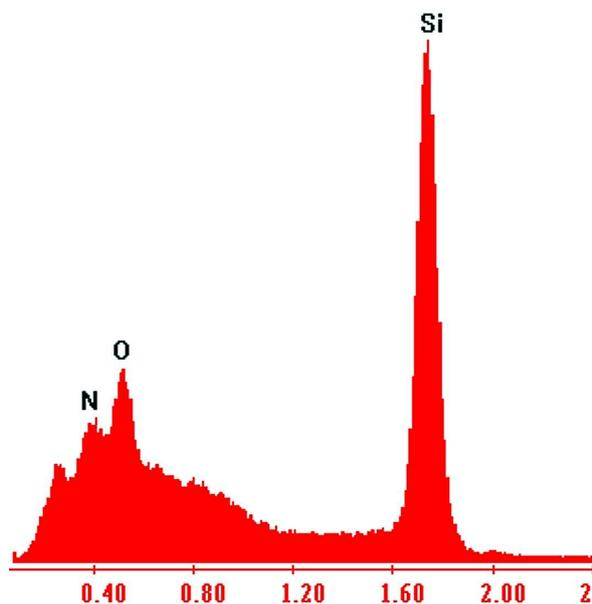
Fig. 7. The EDX spectrum of a typical oxide/nitride film with similar amounts of nitrogen and oxygen. Electron beam energy: 5 keV and the detection take-off angle  $35^\circ$ .
