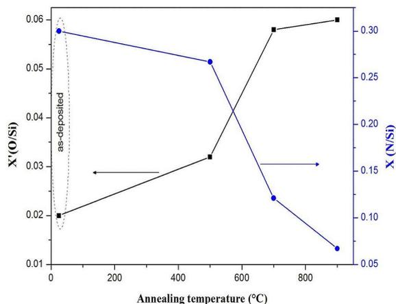
Fig. 8. Correlation between O/Si and N/Si with annealing temperature determined by EDX in oxide/nitride film oxidized at  $950^\circ\text{C}$  during 3 hours. The  $\text{SiN}_x$  films were deposited by PECVD with  $R = 6$ .
