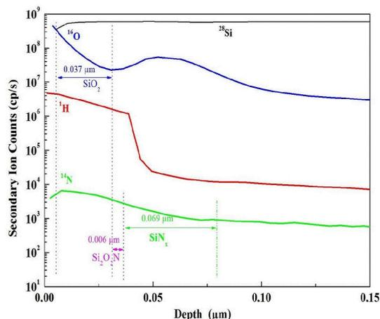
Fig. 1. Depth profiles of Si, O, N and H in an ON structure annealed at  $700^\circ\text{C}$ .
